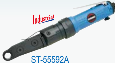
ST-55592A Air Ratchet Wrench (Rear exhaust) Capacity: 10~14mm, 1/2", 9/16" Hex Bolt
