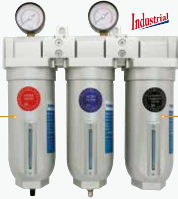
SA-2354A 1/2" Triple-stage Air Filter (Sintered Filter, Fine Filter and Activated Charcoal Filter)
