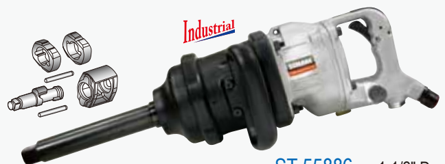
ST-55883 1" Dr. ST-55883-8 1" Dr. W/8" Ext. Anvil Twin Hammer Torque: 3,388Nm (2,500 ft-lb)
