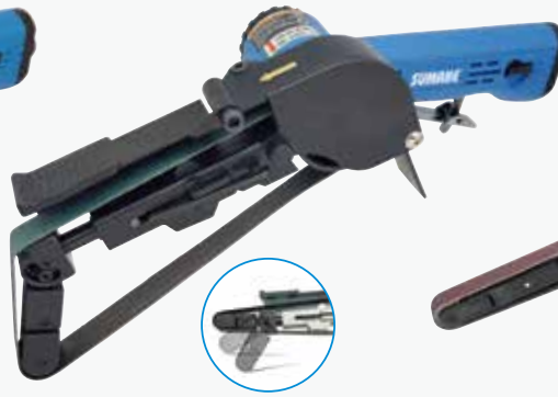
ST-BS111G Iron Pulley ST-BS112G Rubber Pulley 55° Bendable Air Belt Sander With 2pcs Belt (20x520mm, #80, #100) Speed: 16,000 r.p.m.
